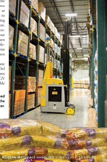
Del Monte relies on more than 30 fork-equipped AGVs for putaway and pallet picking in the distribution center.
