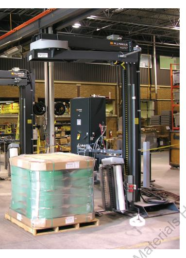
Stretchwrapping is the most frequently used method to unitize a load. Whether being applied manually, semi-automatically or automatically (shown here), film is stretched during the wrapping process then contracts to create the force needed to secure the load.
