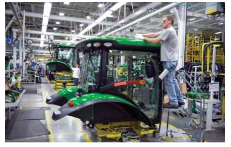
serve as a flexible mobile assembly line, routing the cabs through as many as 12 assembly stations before a finished cab is delivered to the final tractor assembly line.
