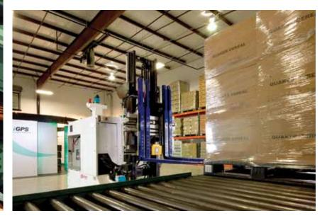
materials handling systems. One manufacturer has installed RFID readers on its palletizing line. After manufacturing, the unit load is automatically palletized, stretch-wrapped and labeled with a license plate bar code label (LPN) that identifies the product on the pallet. The LPN is associated electronically with the RFID serial number on the pallet and written to the warehouse management system (WMS) database.
