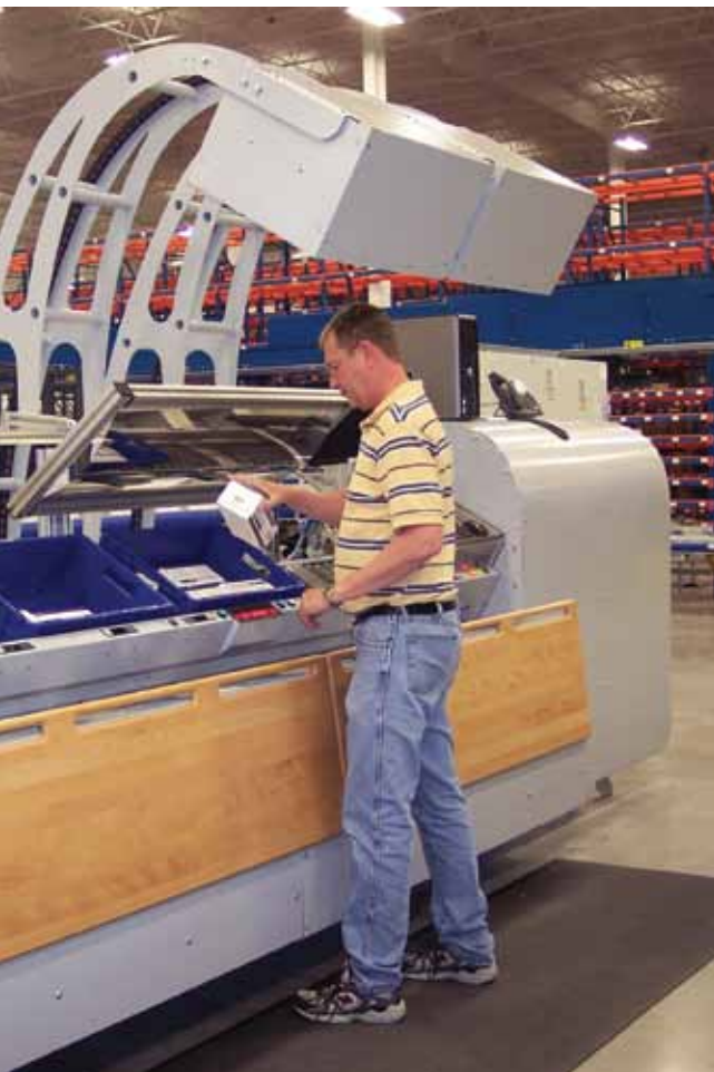
Goods-to-person solutions deliver slow- and medium-movers to a workstation for picking, minimizing the time an associate spends walking.
