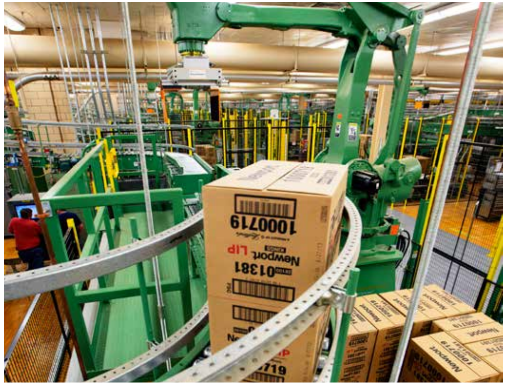
Accuglide accumulation conveyor from Intelligrated carries cases into position for palletizing.
