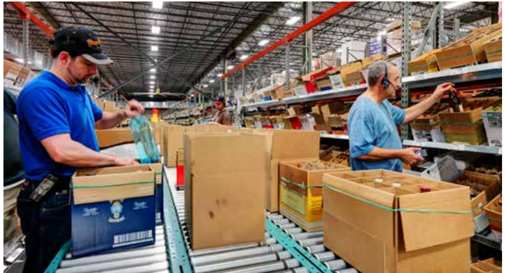
Datria Voice manages complex split-case order picking on the 300-foot bottle picking conveyor line.
