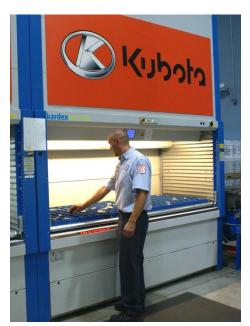
Much of the efficiency from AS/RS equipment comes from replacing substantial amounts of picker travel and handling with a high-density, "goods-to-person" environment in which one or two pickers at a workstation follow pick-to-light instructions to rapidly pick orders. Of course, in many DCs, goods from AS/RS zones need to join up with goods picked from other areas of the warehouse.
