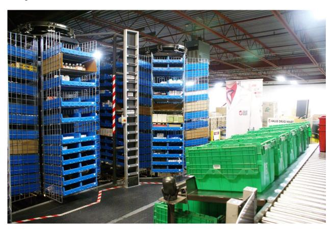
The carousels are an efficient way to pick goods because they rotate to bring the goods that need to be picked to the picker, while Power Pick Global controls the carousels and manages carousel inventory, is smart enough to coordinate batch picking as order requirements come down from the WMS.
